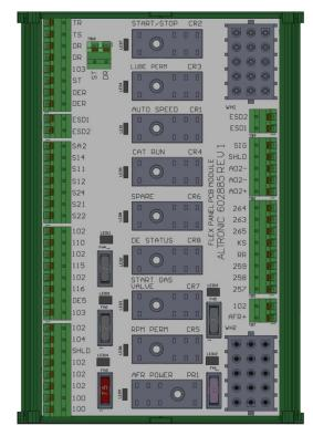
The PCB is equipped with springloaded terminal blocks, relay sockets, automotive style fuses and two harness connections.
