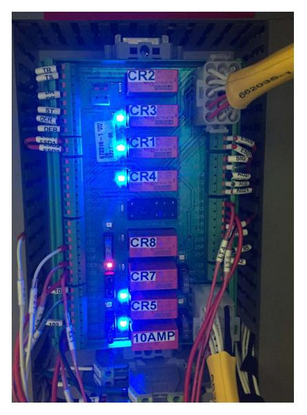
PCB installed in a panel during the QC process. One fuse has been removed to show the red LED. This is the same as if a fuse was blown.
